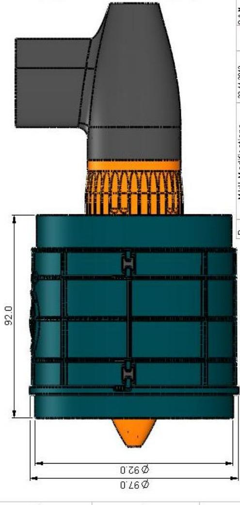
NOTE: 1. INSIDE DIAMETER OF MOTOR TUBE IS 39.1mm TO SUIT NEUMOTORS 1512-1515 SERIES THIN CASE MOTORS OR HET 700 SERIES MOTORS. MOTOR SHAFT SIZE TO BE 5mm.
